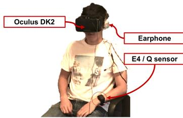
**Figure 4: System Apparatus**
